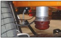
Remove the rubber bump stop by pulling the rubber bumper away from the metal plate.
