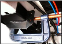
There must be no contact from the bracket on the outside of the chassis. So use a G-Clamp to hold the Upper bracket into position.
