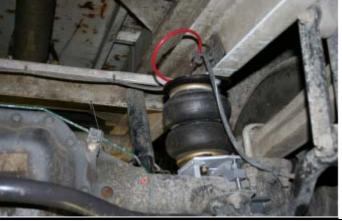
Check that the air spring assembly will not interfere with any other part of the vehicle during normal use.
