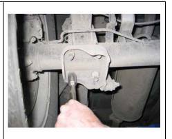
Tighten the upper bracket to the bellows. Using the bolts that held the bump stop in place, bolt the upper bracket to the chassis frame as shown in picture.
