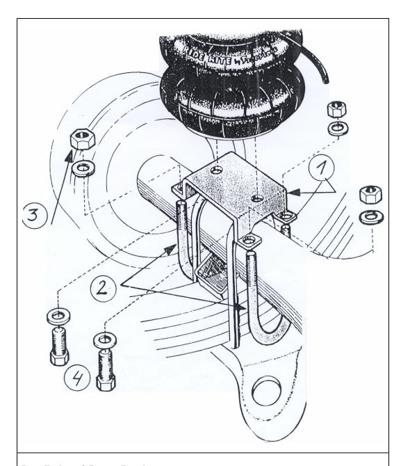
**Installation of Lower Bracket:**Connect the lower bracket to the air spring and bolt it onto the axle / spring by using the supplied U bolts.
