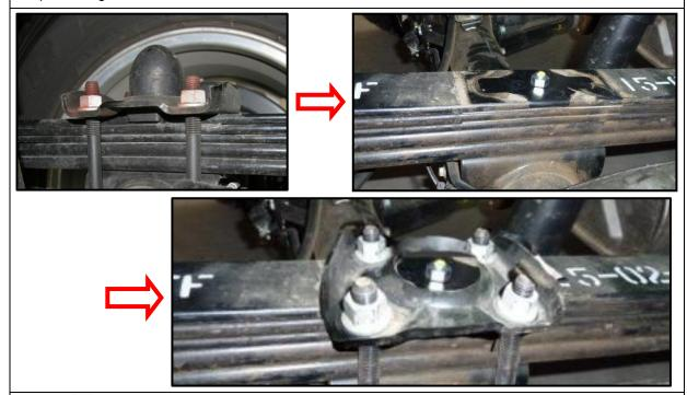
🔰 Step 3: Pre-Assemble Air Spring & Upper Bracket
